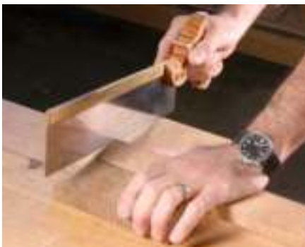
Advance on two fronts. When you mark your cut line on the face of your work, wrap it around the board's edge as well. Then saw by advancing on two lines whenever you can. This greatly improves accuracy.
