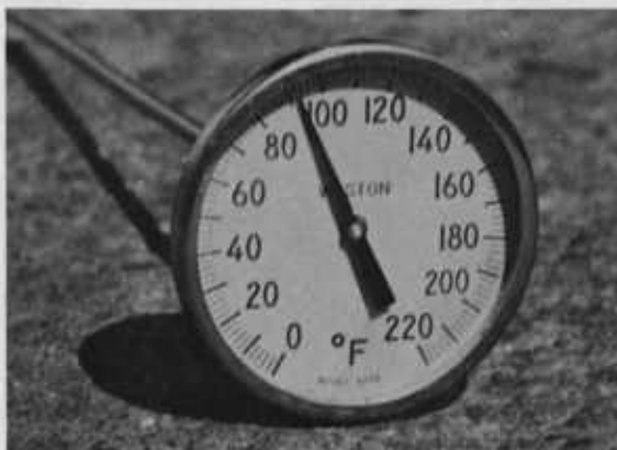
Figure 8.—Dial-type thermometer useful in monitoring dehydrator temperature
